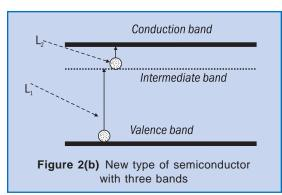
tron to the intermediate band and then up to conduction band using another low-energy photon. A high-energy photon is represented by H in Figure 2 (a) whereas, two low-energy photons are represented by L1 and L2 in Figure 2 (b).
